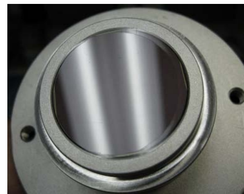
Alta U16M camera with fiber optically bonded CCD
